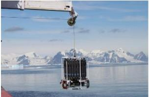
**Figure 2.** CTD cast in Ryder Bay near the British Antarctic Survey (BAS) Rothera Base.
